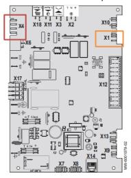
In red: Fan supply cable 230V → connector X4 on CU-HW-01 (v2.01) PCB In orange: Fan control cable → connector X1 on CU-HW-01 (v2.01) PCB
